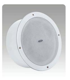
The built-in 5" speaker driver is designed of wide frequency response 110-14.5kHz, power output is 3w, 6w & 9w. The metal grille, metal baffle and metal back cover are in attractive white color.
